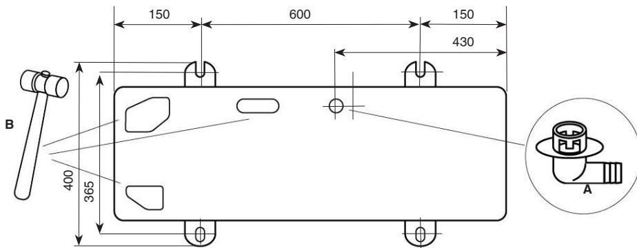
In case of draining through the drain pipe, attach the drain nipple (A) and use a drain hose with an inside diameter of 16 mm (to be provided). In cold outside temperatures when the drain pipe can freeze up, ensure that drainage is not obstructed.
